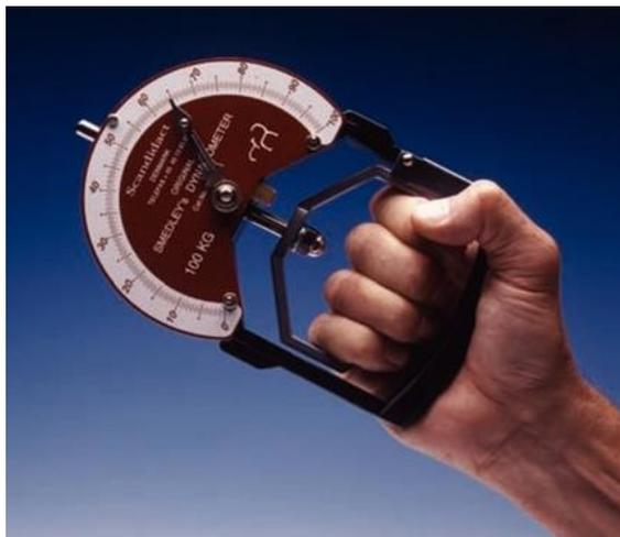
The Smedley's Dynamometer (TTM, Japan or Scandidact, Denmark). After adjusting the device (grip gauge) to suit the respondent's hand and positioning the respondent correctly, the respondent was asked to squeeze the dynamometer as hard as (s)he could for a couple of seconds. Three values were recorded for each hand, starting with the non-dominant hand alternating between hands.
